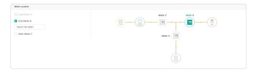
e. Tick on the Export Power Limit function to enable the export control. Input the limit value and click "Finish" to complete the station creation.
